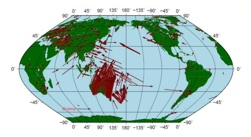
**Figure 1.** The distribution of APREF CORS network along with the IGS core stations. The arrows represent the GPS-derived velocity field.
